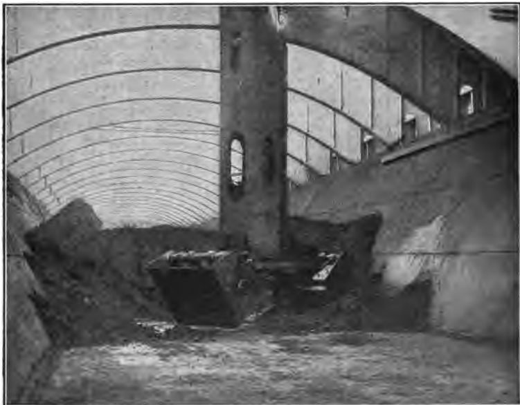
FIG. 170.—Grab buckets of Hewlett automatic ore unloader lifting cargo from the hold of one of the Great Lake boats with its continuously open decks. (Wellman Seaver Morgan Co., Cleveland.)
